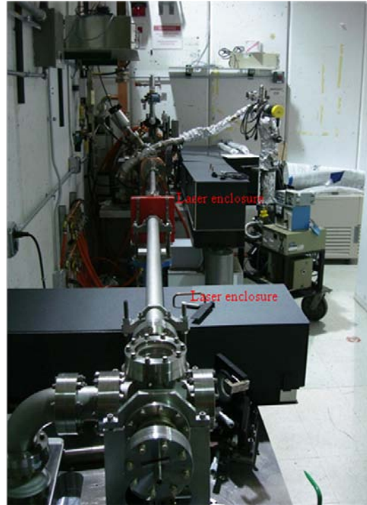
(left) UED photocathode, solenoid, sample chamber and beam diagnostics, (right) schematic of UED system including laser enclosure
